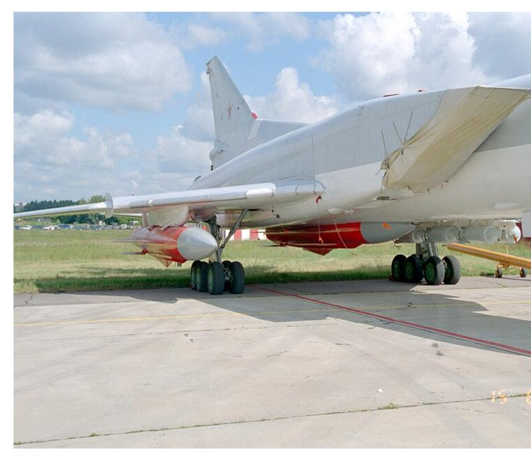
We see one Kh under the starboard wing and another in a conformal [ie half-buried] position under the fuselage...the port wing would carry a third Kh...
