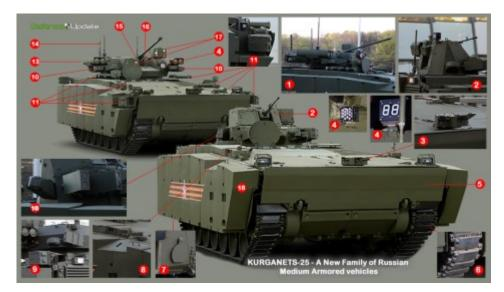
As with the Armata T-14 tank, the T-15 IFV is protected by four types of armor. It uses the same navigation equipment and optoelectronics, the same engine, a similar central fire control, etc. The BTR/BMP Kurganets-25 IFV is for infantry and elite mountain troops; it is powered by a 800hp engine. It has a 3-man crew and can carry eight infantrymen.
